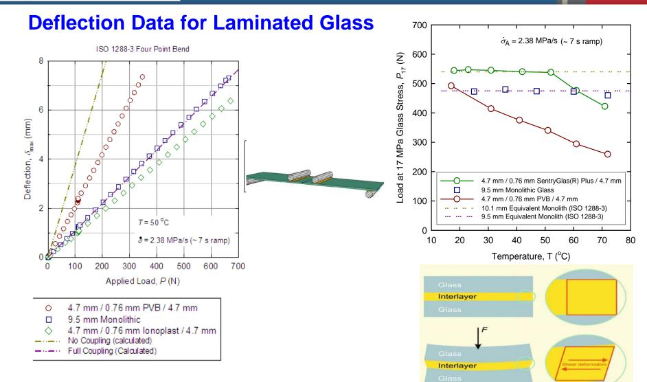
Laminates with SentryGlas<sup>®</sup> develop least deflection at a specified applied load -Note thickness differences
